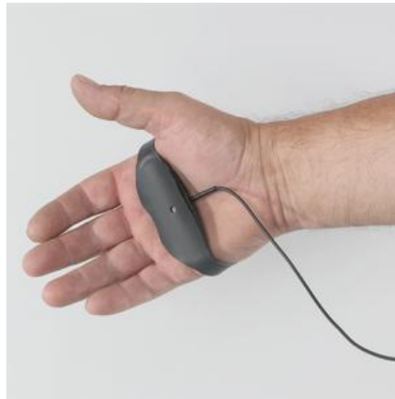
Photo 2 Hand-arm vibration adapter with tri-axial MEMS sensor installed
